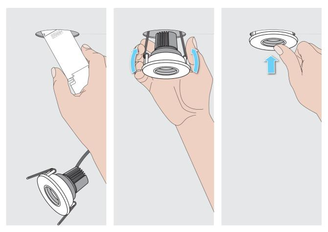
Insert the driver and the back of the downlight through the Ø64mm hole.
