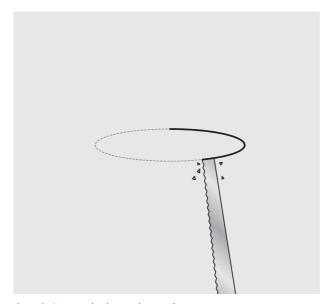
Cut Ø64mm hole in the ceiling.
