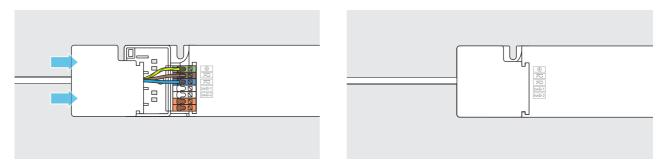
Clip on any strain relief clips and terminal cover/lid.
