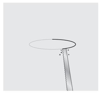
Cut Ø115mm hole in the ceiling.
