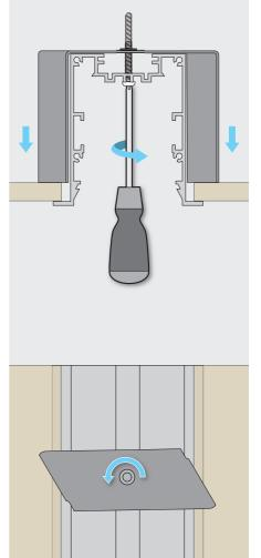
Ensure luminaire is tight in the ceiling and not loose.
