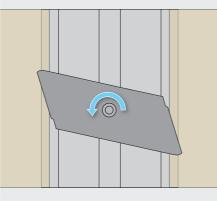
Using screwdriver, push screw up and begin to tighten screw.
