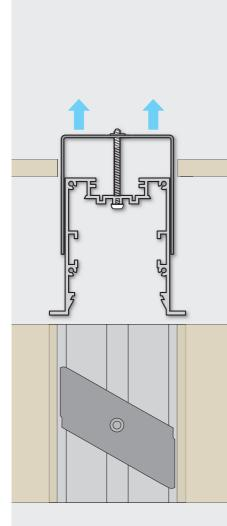
Insert Millie in to ceiling cut out with brackets tight against luminaire.
