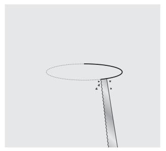
Cut Ø82mm hole in the ceiling.
