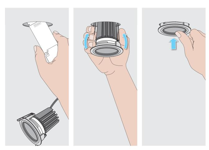
Insert the driver and the back of the downlight through the Ø82mm hole.
