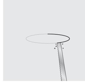
Cut Ø160mm hole in the ceiling.
