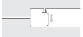
Clip on any strain relief clips and terminal cover/lid.
