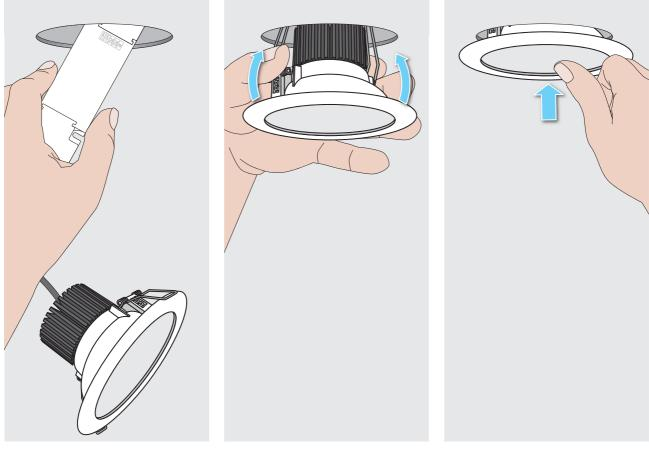
Insert the driver and the back of the downlight through the Ø160mm hole.
