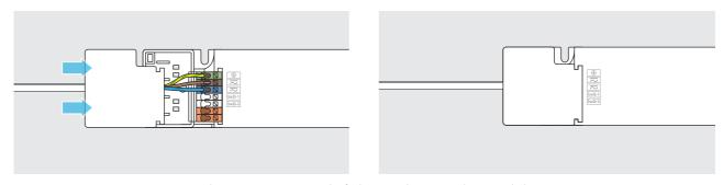
Clip on any strain relief clips and terminal cover/lid.
