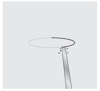
Cut Ø95mm hole in the ceiling.
