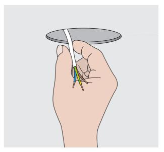
Pull the cable through the hole and connect to the driver.
