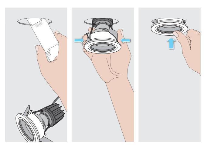
Insert the driver and the back of the downlight through the Ø95mm hole.
