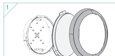
Remove the bezel (if aplicable) and diffuser from the base. If required remove any screws from the diffuser.
