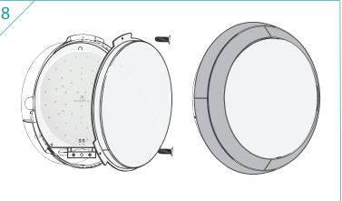
Once wired up carefully fix the gear tray / pcb, diffuser and bezel back onto the base, securing with screws when required.
