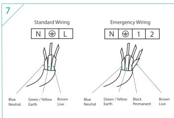
Once correctly wired up test the luminaire before fixing the diffuser and base back on.
